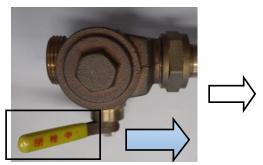
『閉栓中』(closed) is shown on the lever.
